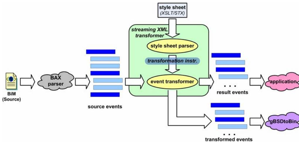
Figure 6 — Architecture of Streaming Transformer for BiM.
